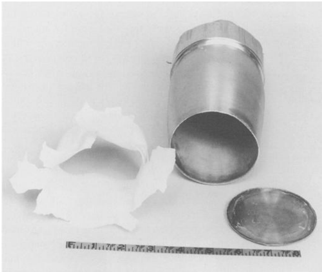
FIG. 1—Main electrolysis "cold fusion" cell with detached base (inner surface shown) and ripped Teflon insert. The main cell impacted the head of the victim and caused the fatality.
