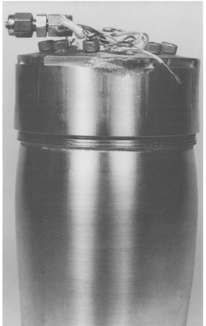
FIG. 3—Side-view of the electrolysis cell. Note bulge below the threaded metal. Internal pressure estimated at 300 atm distorted the 0.2-cm thick, stainless-steel vessel from its initial configuration of a right-circular cylinder.
